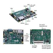
Designed for applications such as IoT/M2M-related, industrial control, self-serve terminal, digital signage, POS and kiosk, the Axiomtek CAPA840 allows dual views through multiple display outputs of HDMI, LVDS and VGA. Additionally, the compact embedded SBC adopts a ZIO connector and has two PCI Express Mini Card slots for flexible custom configurations. It features wide voltage DC-in +12V to +24V to make power input more flexible.
