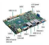
Axiomtek is pround to announce the CAPA318, a fanless 3.5-inch embedded motherboard, featuring Intel® Pentium® processor N4200 or Celeron® processor N3350 with low power consumption. The CAPA318 can be ideally applied to extended temperature environment from -20°C to +70°C. -read more-
