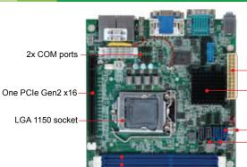
\_\_\_\_ 24 Pin ATX power connector
